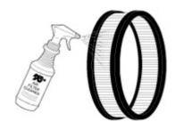
Spray K&N air filter cleaner liberally onto the entire element and let soak for 10 minutes.
