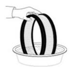
Large K&N elements can be rolled or soaked in a shallow pan of K&N air filter cleaner. Remove immediately and let sit for approximately 10 minutes.
