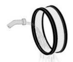
Rinse off the element with low water pressure, tap water is OK. Always flush from the clean side to dirty side. This removes the dirt and does not drive it into the filter.
