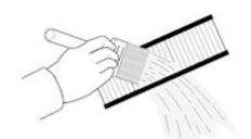
Tap the element to dislodge any lodge embedded dirt, then gently brush with a soft bristle brush. (Note: If complete cleaning is not practical at this time, re-oil the element and re-install in your vehicle.)
